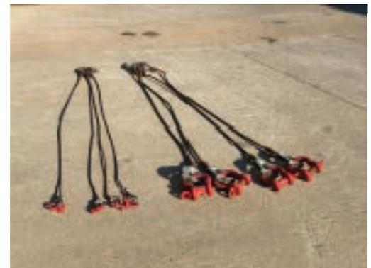
\*\*\* All rigging is certified and tagged with size, length, max load, serial number, and date of load test \*\*\*
