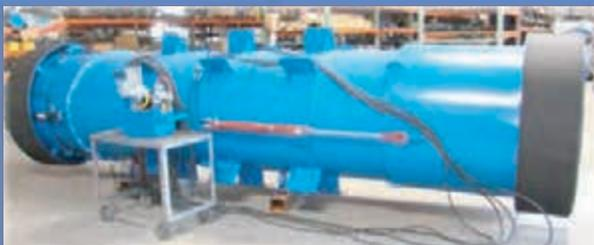
**66" Hydraulically Actuated Telescopic Flow Diverters** used to dry up a structure. Diverters are steered into place remotely with included hydraulic control panel.
